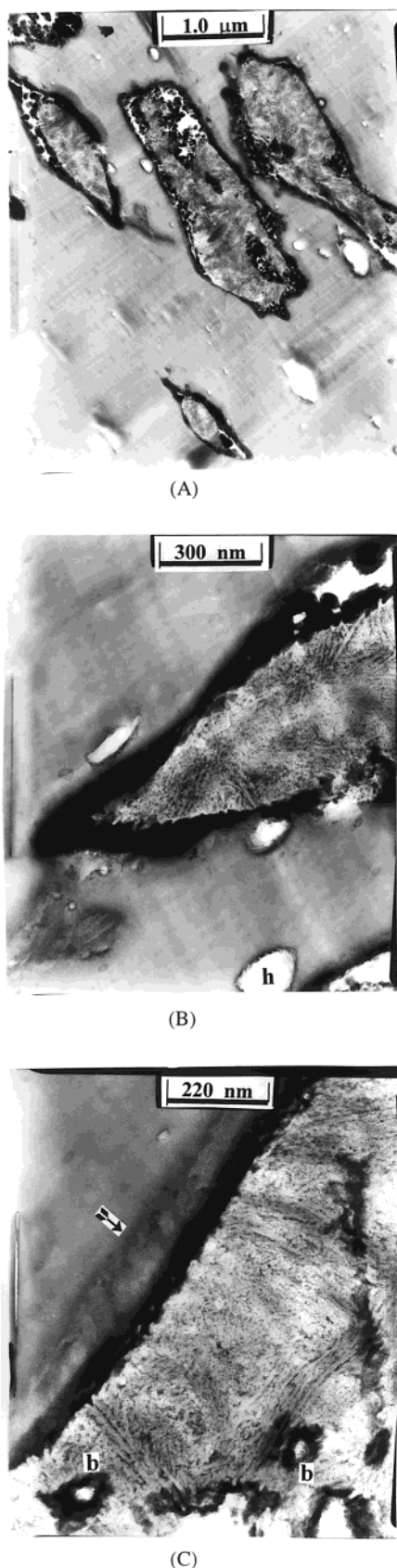
Figure 5. TEM micrographs of the PS/HDPE/SBS (72/18/10) blend transferred from the hot press to boiling water and cooled naturally: (A) a view of PE particles and the surrounding interfacial layers; (B) and (C) the detailed structure of the interfacial layer.
